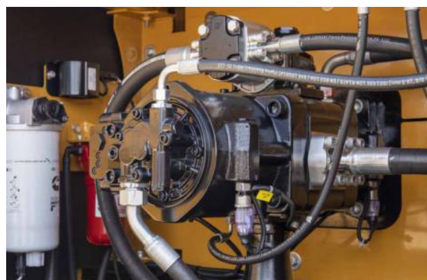
Main valve model: KMX15RB Rated flow: 300 L/min Rated pressure: 37.7 MPa
