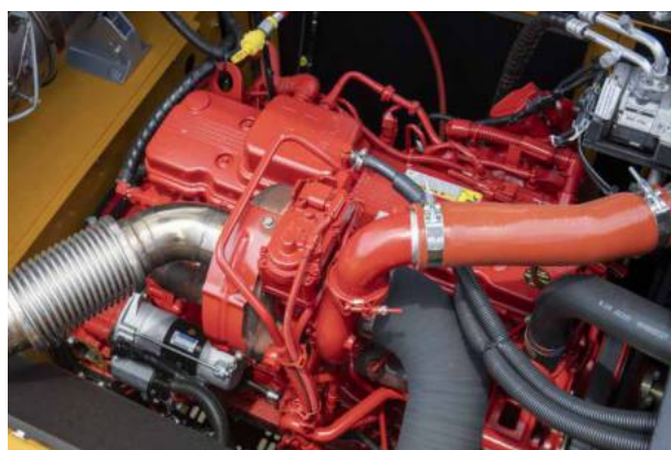
Engine model: QSB6.7 Engine power: 129KW/2200rpm Displacement: 6.7 L
