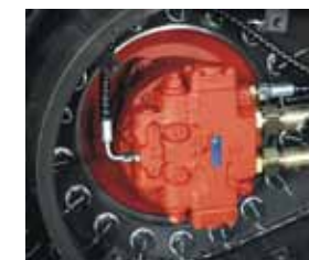
SY335C travel motor driving force increased to 274KN.
