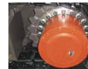
SY365C travel motor driving force increased to 320KN.
