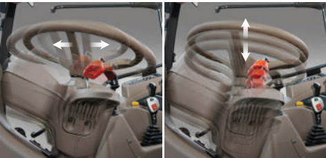
Tilting and telescopic steering The steering wheel can be adjusted according to the driver's physique and preferences. (Tilting 24 degrees, Telescopic length 50mm)
