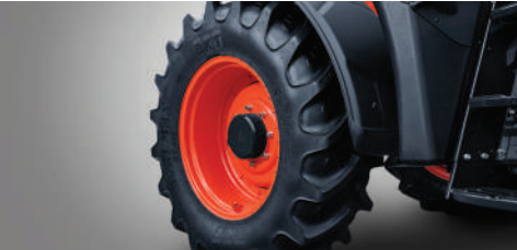
Radial tires Radial tires allow for comfortable driving with low vibration, and their strong traction is optimized for towing operations. (Front: 420/70R28, Rear: 520/70R38)
