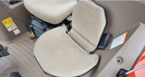
Auto folding auxiliary seat Transportable with co-passengers to the workplace, enhancing boarding convenience with an automatic folding seat.
