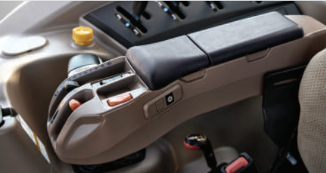
Electronic armrest The arm rest can be moved front and back and the lever and switch can be operated conveniently for easy 3-point hitch control of the rear.
