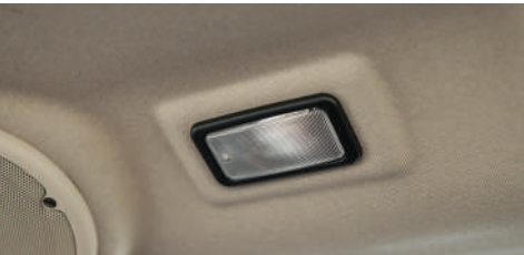
Auxiliary interior lights Separate auxiliary interior lights that shine upon the work lever offers better vision of operating levers/switches during night work as well.
