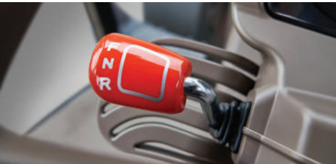
Power shuttle Conveniently shift between forward and reverse without pressing the clutch pedal, using only lever operation.
