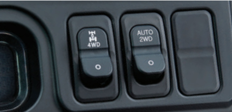
4WD switch When off, it switches to 4WD and when on, it switches to 2WD automatically, enhancing parking and driving convenience and the switch can be pressed during driving to switch to 4WD easily.
